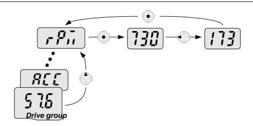
How to monitor Motor rpm in Drive group when the motor is rotating in 1730 rpm.
